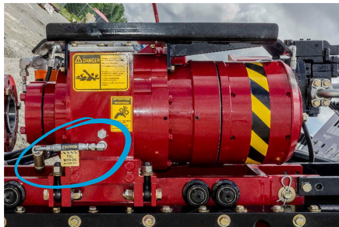
Figure 20 Oil level view port the drill head.
