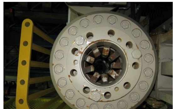
Figure 59 Nine grease points on the top the of the drill head chuck.
