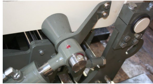
Figure 55 Top of the hydraulic piston that raises the mast on each sided of the base.
