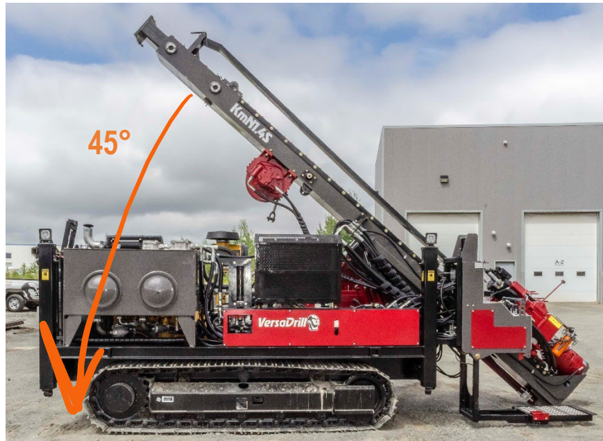
Figure 15 Drill with mast at 45 degrees.
