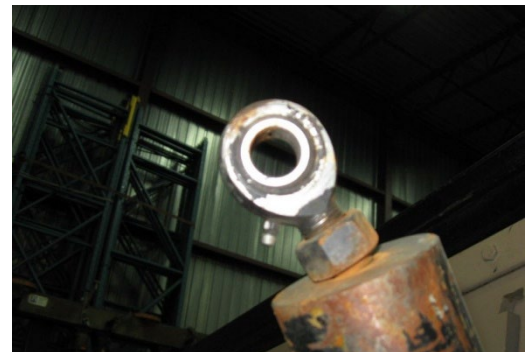
Figure 61 Grease the eye bolt on the tip of the support pole (2 total).
