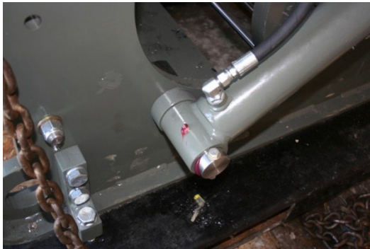
Figure 56 Bottom of the hydraulic piston that raises the mast on each sides of the base.
