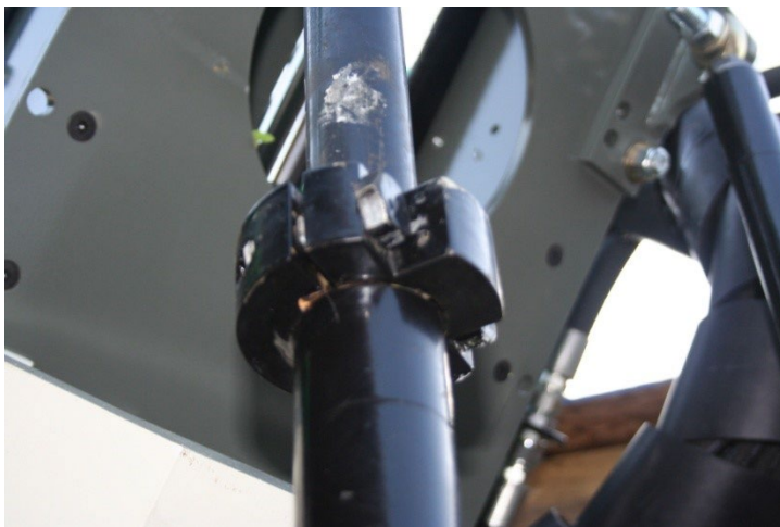
Figure 40 Adjustment bolts on the poles.
