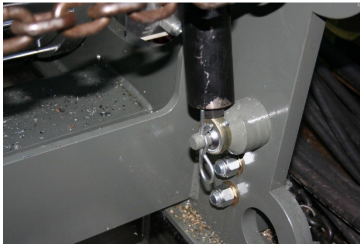
Figure 39 Poles bolted to the base.
